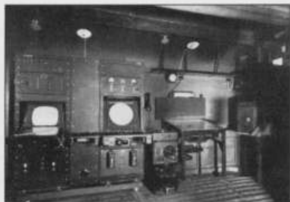
Left: Common T&R aerial of mobile GCI (Type 15). Right: Interior of typical mobile GCI vehicle. The left-hand display (similar to the range tube of CHL) has additional facilities for estimation of target heights. PPI is on the right.
