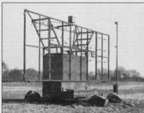
Left: Common T&R aerial of mobile GCI (Type 15). Right: Interior of typical mobile GCI vehicle. The left-hand display (similar to the range tube of CHL) has additional facilities for estimation of target heights. PPI is on the right.
