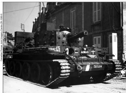
A Royal Marine Centaur in Courseulles, late on 6 June, still sporting its wading equipment. Eight of these SP howitzers from "S" and "T" Troops, 2 RMAS, were assigned to help the Regiments with indirect fire controlled by FOCs from 13th RCA. "S" Troop appears to have landed only two guns, while "T" Troop had three of its four SPs disabled by track damage on the beach. Nonetheless, Centaur fire - even on a small scale and often in an assault gun role firing direct - was crucial to the clearing of Courseulles, and other strongpoints along Juno beach, on D-Day.
